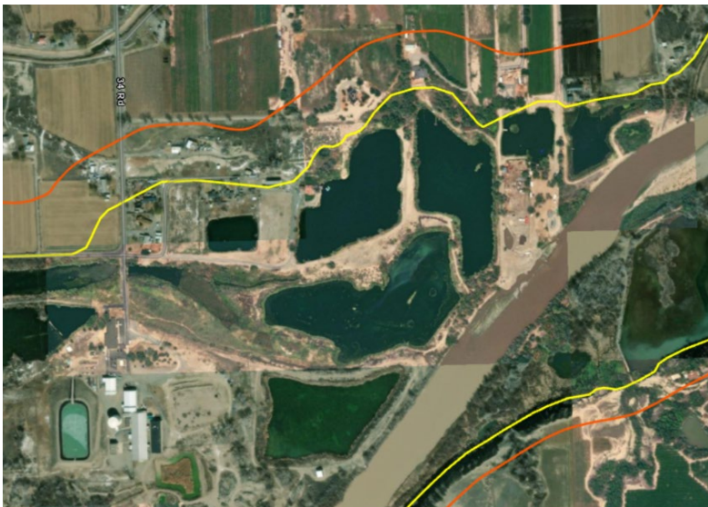
Figure 6-12. Gravel ponds located within the Clifton area constrain flood flows and channel migration.
