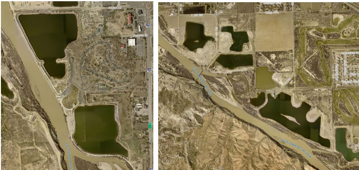
Figure 6-19. Examples of gravel ponds constricting the floodplain of the Colorado River in the Fruita area.
