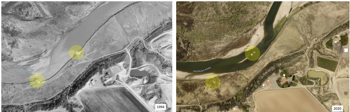
Figure 6-7. Bank armoring structures flanked by a migrating Colorado River. Located at approximately 30 ½ Road.
