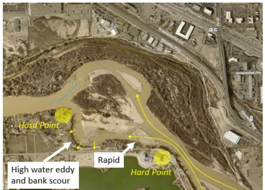
Figure 6-18. Arrested down valley channel migration and artificially forces southward migration at Dike Road near Connected Lakes State Park.
