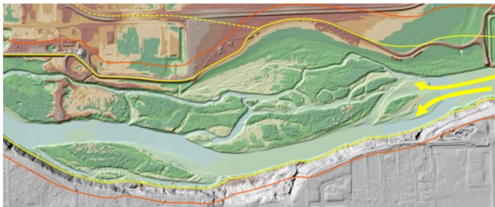
Figure 6-16. Channel expansion and deposition at inlet of the River Park at Las Colonias.
