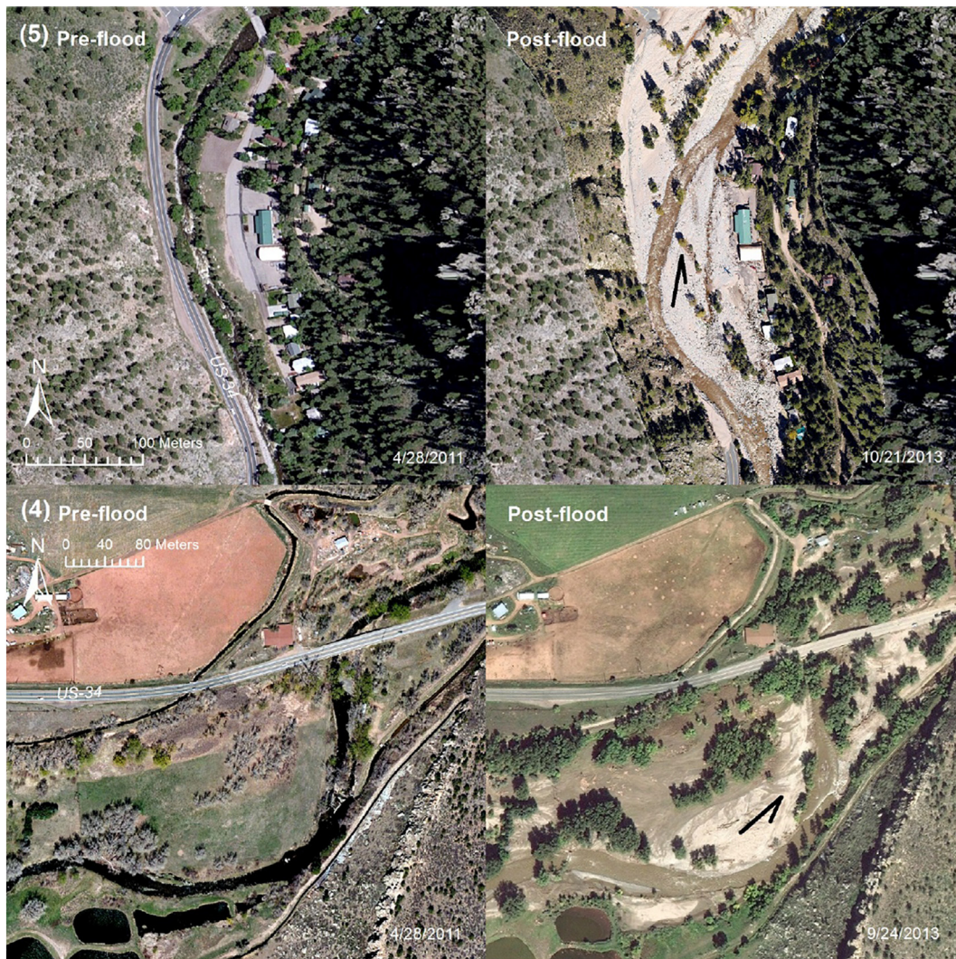
Fig. 3. Examples of geomorphic change for classes 5 and 4, with paired pre- and post-flood imagery. The upper pair illustrates class 5 geomorphic change, with channel adjustment and the resulting elimination of the armored US-34 roadway embankment along the Big Thompson River. The lower pair, also for the Big Thompson River, illustrates class 4 geomorphic change with the channel substantially widening for a majority of the reach length but not shifting or avulsing. Sediment deposition on the floodplain surface is also apparent, but woody riparian vegetation was not substantially impacted otherwise. Imagery sources: ArcGIS Online and DigitalGlobe. (Note: dates are month/day/year.)
