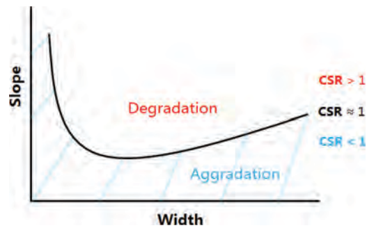
Figure 4-10. Family of width and slope combinations which provide continuity of water and sediment.
